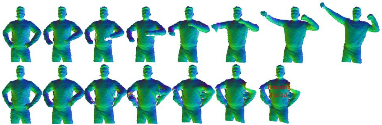
Fig. 7. Demonstration of using model reinitialization mechanism to handle close-to-open topology changes and fast motion. Top: the reconstruction by our approach. Bottom: the reconstruction by DynamicFusion [14] (our implementation).
