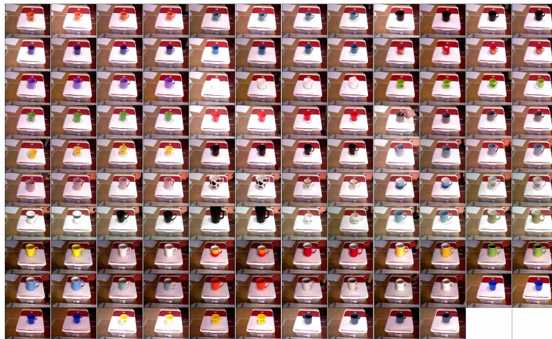
(b) Image of the mug shelf after running the kPAM pipeline. Red images indicate trials where no image of the final placement was captured due to an upstream failure of the pipeline causing the trial to be aborted.
